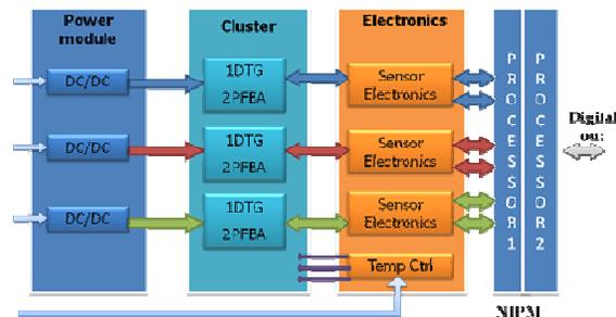
Fig. 1 System Configuration
