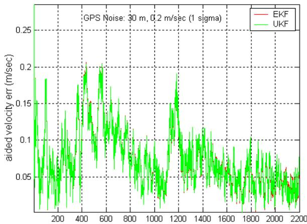
Figure 5: Aided velocity error with noise in GPS and INS data
