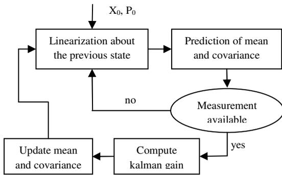
Figure 2: Extended Kalman Filter Algorithm
