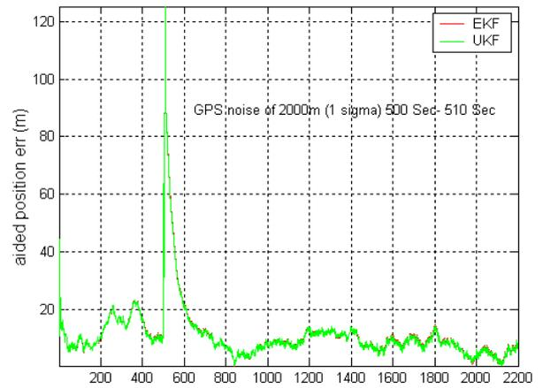
Figure 8: Aided position error with burst of noise in GPS data
