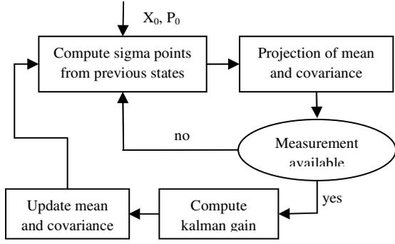
Figure 3: Unscented Kalman Filter Algorithm
