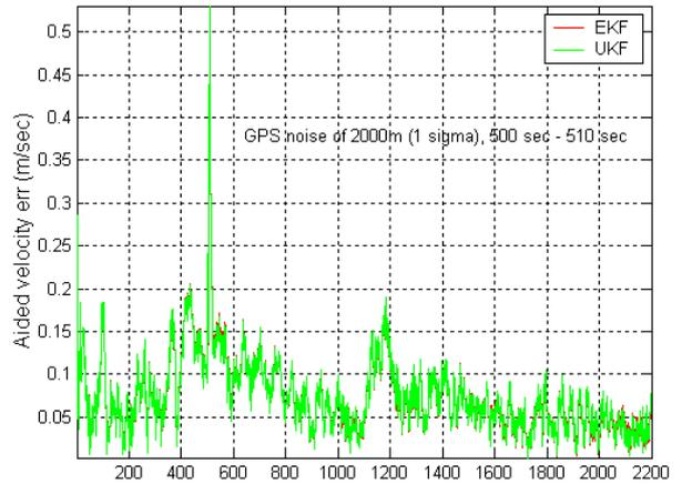
Figure 9: Aided velocity error with burst of noise in GPS data
