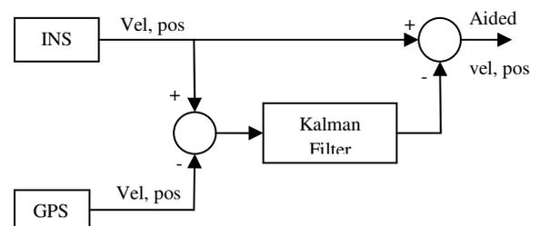
Figure 1: Block Schematic of GPS aided INS
