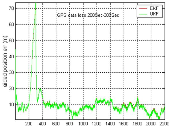
Figure 6: aided position error with loss in GPS data
