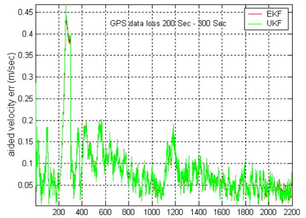
Figure 7: Aided velocity error with loss in GPS data
