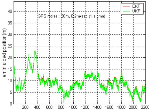
Figure 4: Aided position error with noise in GPS and INS data
